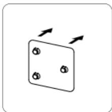
2. Stick the mounting board on the clean surface in the correct direction and press firmly to ensure complete adhesion.
