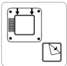
1. Clean and dry the surface where the mounting board will be pasted. Remove the protective film from the adhesive tape on the back of the mounting board.
