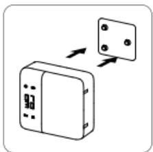
3. After 24 hours, install the main unit on the mounting board, ensuring that it is secured properly.
